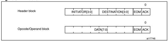
All these blocks are made of an 8-bit payload (most significant bit transmitted first) followed by an end-of-message (EOM) bit and an acknowledge (ACK) bit.
