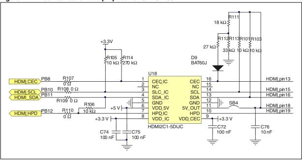
Figure 13. Electrical schematic proposal for STM32100E-EVAL
